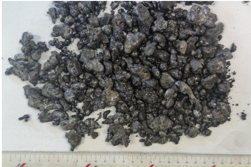
Figure 2. Slag pouring from the EAF and the subsequent slag air granulation at METLEN's pyrometallurgical pilot.
