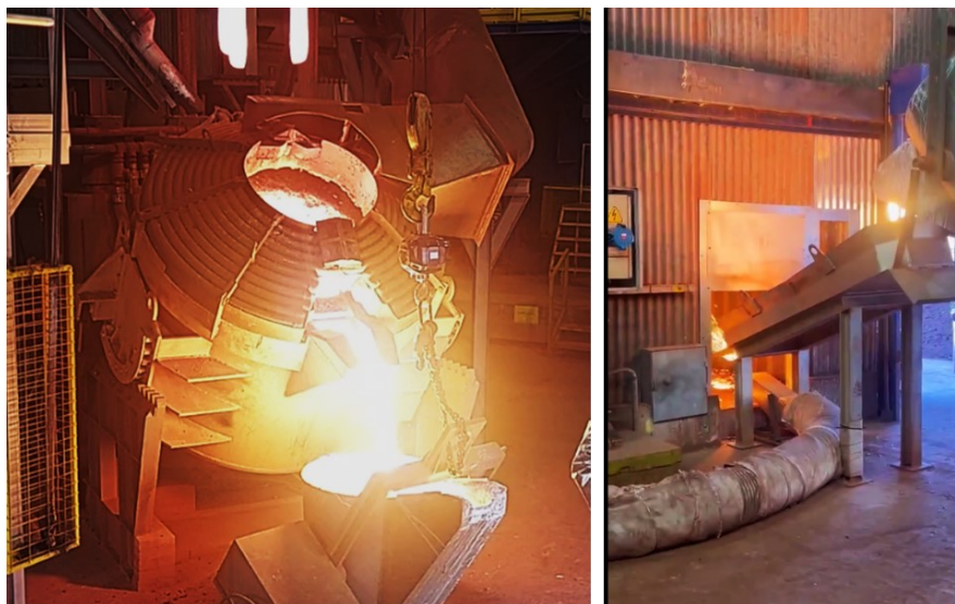
Figure 1. Slag pouring from the EAF and the subsequent slag air granulation at METLEN’s pyrometallurgical pilot.
